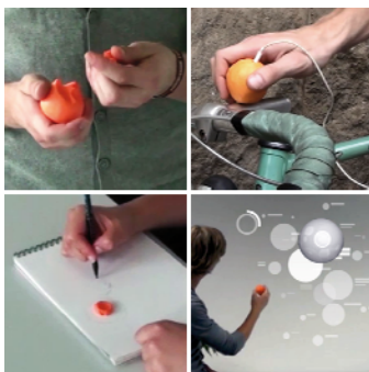
Figure 10: Plasticine used directly as interface for the Kneadable Computer .
